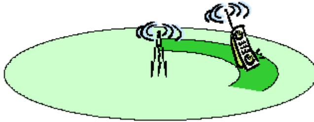
Figure 2.5: Cell-ID with sector and timing advance [1]
