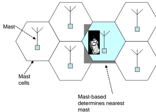
Figure 1.2: Mast-based location
