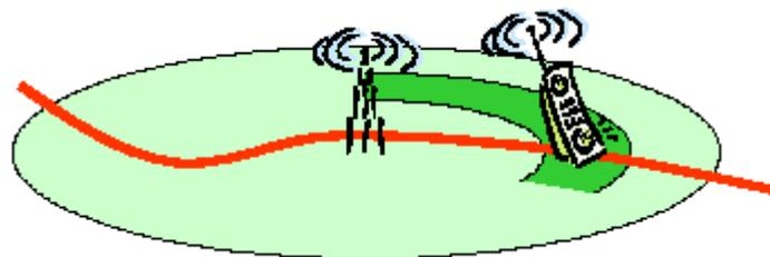
Figure 2.7: Cell site with sector, timing advance and supplementary information [1]
