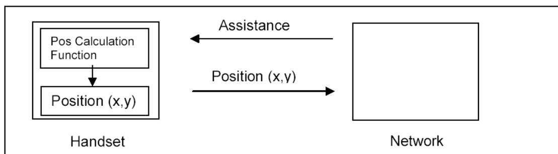
Figure 2.1: Handset based mode
