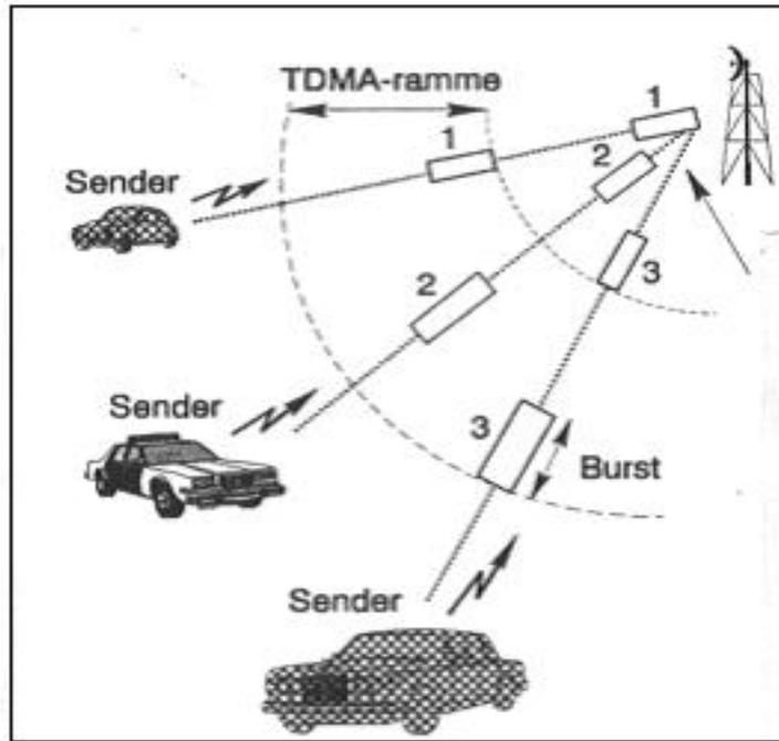
Figure 4.1: The synchronisation of TDMA frames
