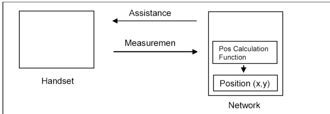
**Figure 2.2:** Handset assisted mode
