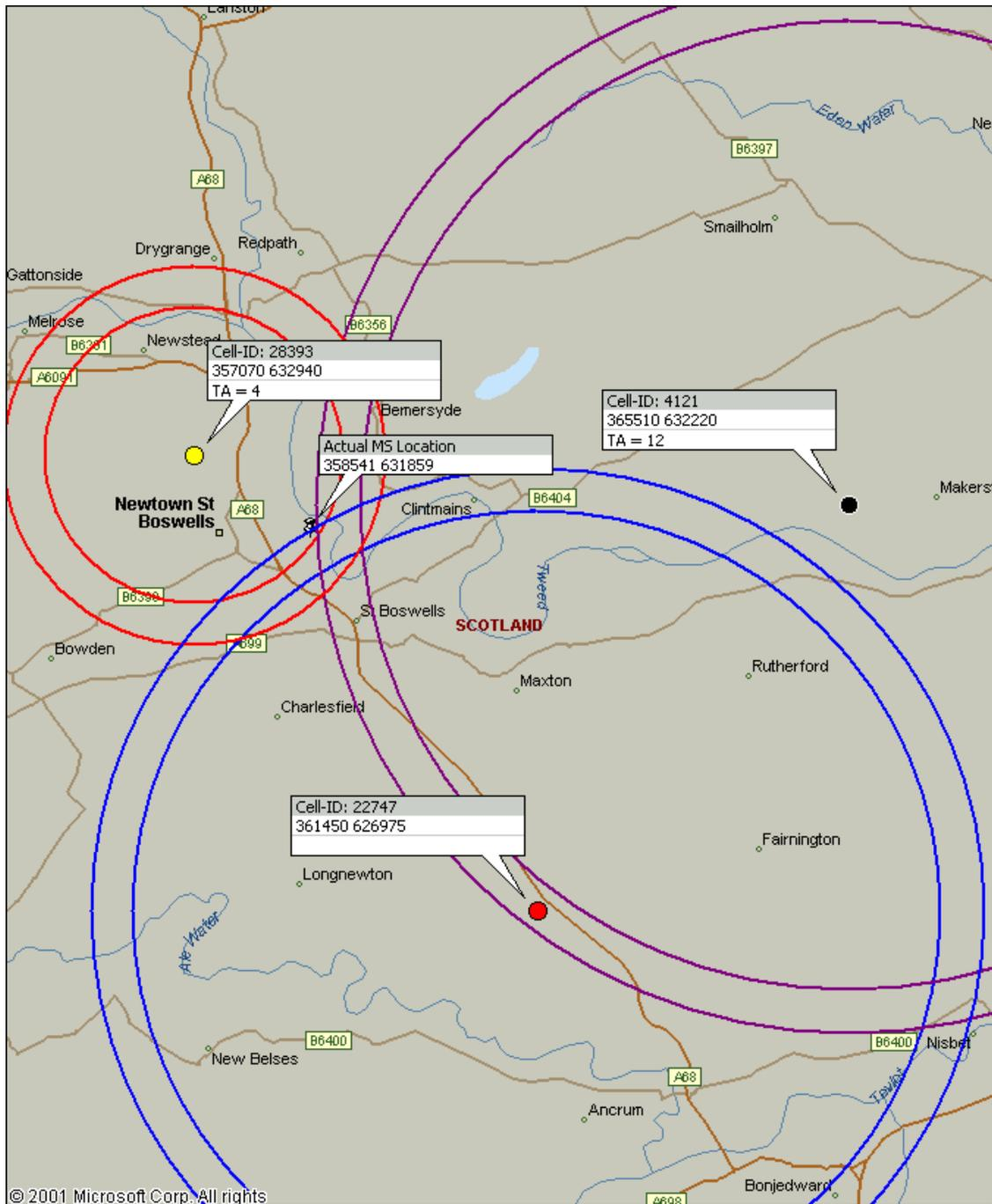
Figure 4.2: Concentric circles for each BS showing distance from MS
